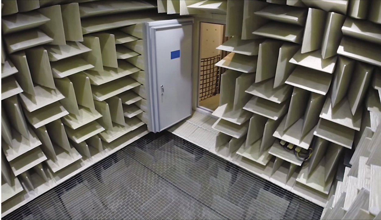
Figure 3. An anechoic chamber. Note the wedges on the inside of the open door and the suspended wire mesh floor. The wedges are 1.2 m (4 ft.) long. (Courtesy of Eckel Noise Control Technologies, Microsoft)
